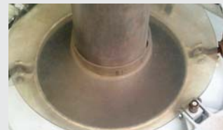
Spill protection during loading
