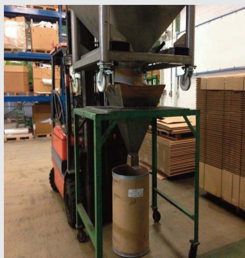
Additional funnels ensure that pellets can't fall out at the sides
