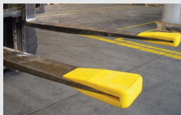
Soft tips on fork lift trucks prevent tearing of bags
